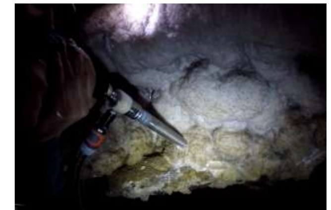
Core-drilling and sampling of gypsum deposits in Provalata Cave
